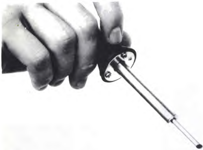
Figure 1. The most important tool for the electronic hobbyist is the soldering iron. This illustration shows a typical hobbyist iron and the correct way to hold it.
